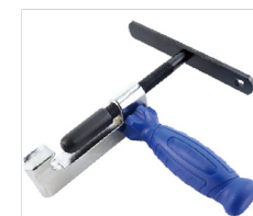
CT-204 Pinch-off Tool In extra strong execution to pinch-off suction tubes on all hermetic refrigeration systems up to 3/8" diameter.
